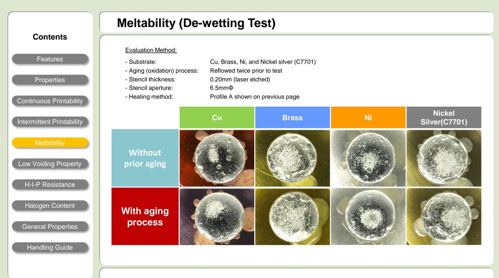
S3X58-HF1000 had good solder spreading and no de-wetting occurred regardless of the metal finish even with the intentionally oxidized finishes.
